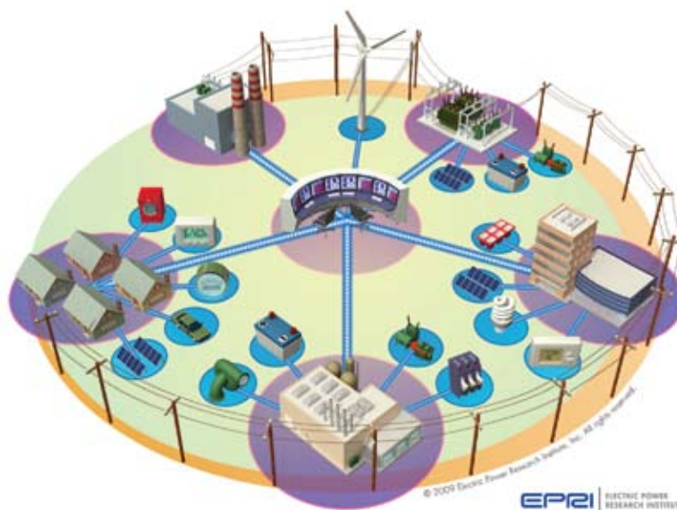
Figure 7: This diagram of a smart grid illustrates in which way local energy sources, buildings and electrical vehicles are interconnected. Source: Utrecht Roadmap To a Third Industrial Revolution
