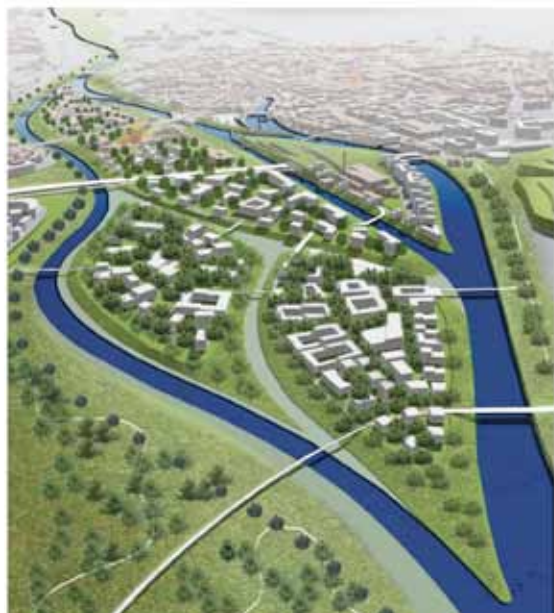
The Dutch office Kuipercompagnons advised to reopen and reuse former riverbeds of the river Warta for water catchment. The illustrations show low and high water level.
